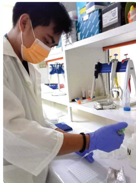
Pipetting supernatant after centrifugation for nanoparticle purification.
